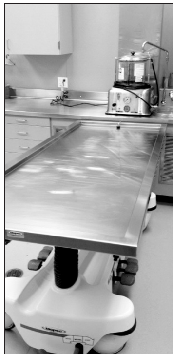
Embalming table set up in the prep room. The foot end is slightly lower than the head end and is over the drain bowl. Notice the draining channel that goes all the way around the table.
